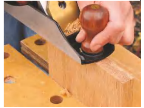
STEP 3. Plane the board ends square, working from each end towards the middle to prevent any splitting
